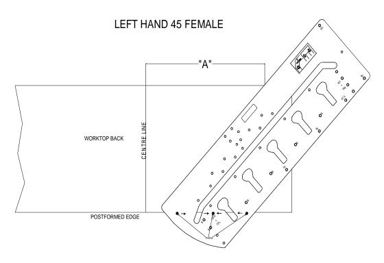
Once both of the female cuts have been made, set the work piece to one side as you will need to trim the back edge, before the worktops are brought together.
