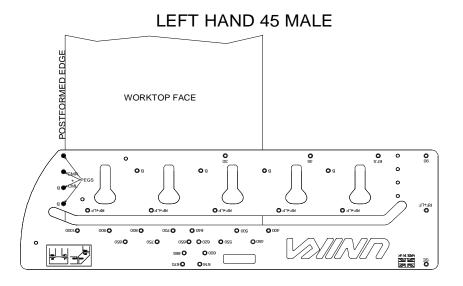
Once the male cuts are complete the two male sections should be offered up to the corresponding sides of the corner section and the parts of the centre piece to be
