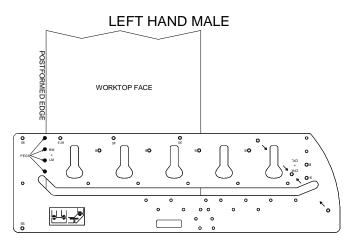
Set the jig onto the worktop as shown and clamp firmly in place. Again, always starting the router from the extreme left of the slot, use the side of the slot nearest to you setting the plunge depth to no more than 10mm per pass, remove the waste.
