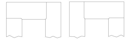
The layouts above are preferable to that below. If however it is necessary to use this construction, careful measurement is required to ensure a good fit.
