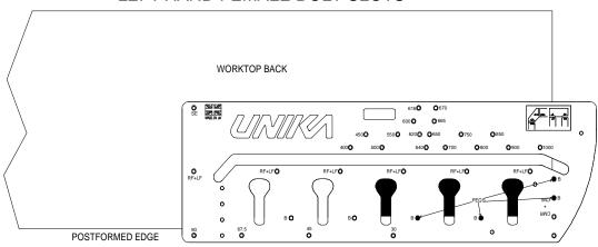
With the worktop face down set the jig in place (jig face up for left hand female bolt slots and jig face down for right hand female bolt slots). Once the pegs are butted up to the edges of the worktop clamp the jig in place using two G clamps, checking the jig has not moved after tightening.
