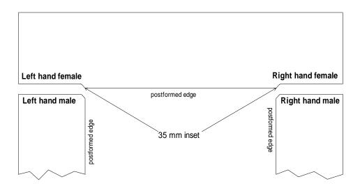
The construction shown above is the easiest to fit and should be used if possible. Alternative layouts are shown on pages 11 and 12 of these instructions.
