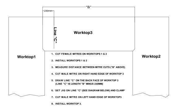
The preferred steps in fitting the setup above are shown as steps 1-8. The measurements must be taken from the edge of the cut mitre. The jig set-up to cut the male mite on the left hand end of Worktop 3 above is shown below.
