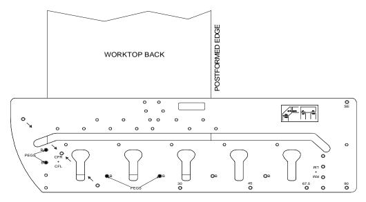
Again with the worktop face down set the jig in place (jig face up for right hand male bolt slots and jig face down for left hand male bolt slots). Clamp the jig in place as before and repeat the routing procedure described on the previous page.
