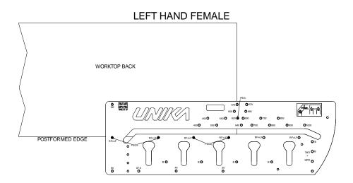
The diagrams above show the female mitre set-up for a 620mm wide worktop, for other work top widths the peg used to set the cut length should be changed.
